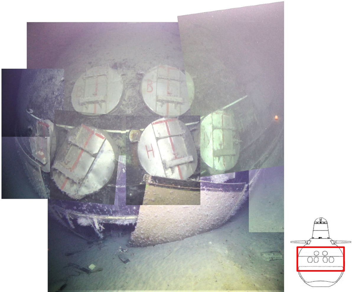
Figure 4.20. View of the bow of Komsomolets showing the plugs installed over the six torpedo tubes by the Russian investigation to Komsomolets in 1994 and the damage to the lower outer hull (Photo composite: DSA/IMR). Red frame on the plan drawing of Komsomolets shows the relative position of the image above.
