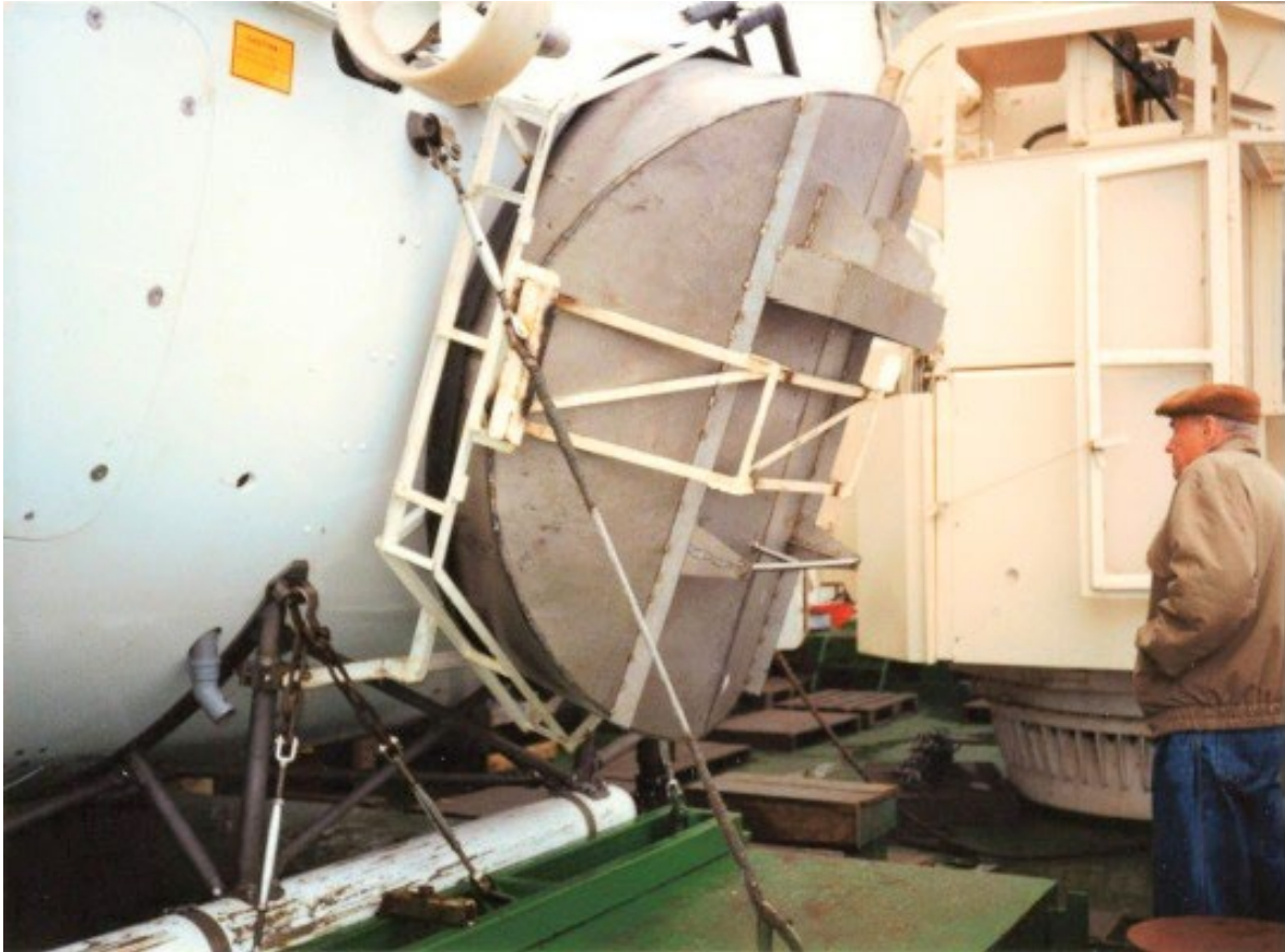
Figure 1.6. Photo showing one of the titanium plugs that was placed over the torpedo tubes by the Russians in 1994. The plug is fastened to the side of one of the MIR submarines used during the 1994 Russian investigation. (Photo: DSA).
