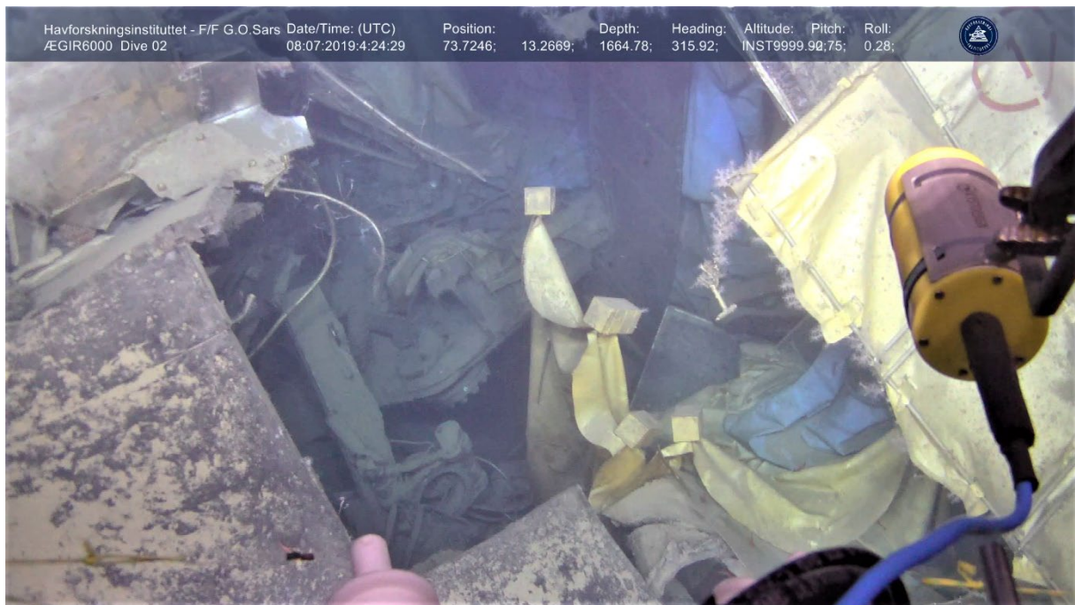
Figure 4.14. View down into the opening in the outer and inner hulls seen in Figure 4.13. The blue and yellow objects are part of the material that was packed into the torpedo compartment during the Russian investigation to Komsomolets in 1994. The yellow instrument in the ROV's manipulator arm is a Geiger counter (Photo: IMR).
