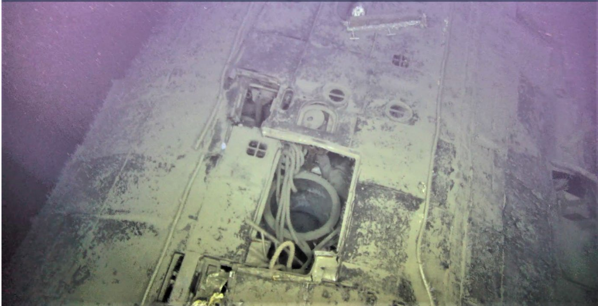
Figure 4.11. Close up view of the forward entrance hatch that led to the torpedo compartment. The outer hatch and coaming were missing, but it was not possible to determine whether the inner hatch was open or closed (Photo: IMR).
