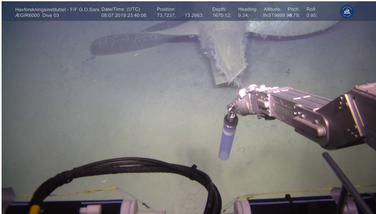
Figure 2.5. Push core being taken next to main propeller (Photos: IMR).
